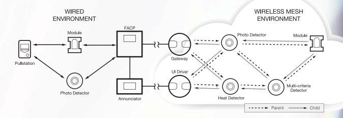
A SWIFT wireless system can use any combination of modules, smoke and/or heat detectors. In addition, both wired and wireless devices can be present on the same fire alarm control panel (FACP), providing an integrated wired-wireless solution for increased installation potential.
